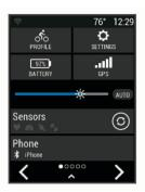
The settings widget appears. A flashing icon means the device is searching for a signal. A solid icon means the signal was found or the sensor is connected. You can select any icon to change the settings.
